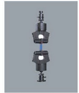
SG-005(#753-051) Max load:1KN Usage: Plastic, thin film, leather etc. tensile experiments
