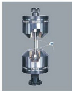
SG-007(#753-071) Max load:600KN Usage: All kinds of metal and non-metal materials tensile experiments
