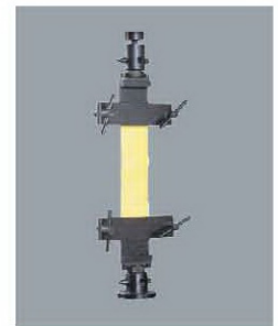
SG-010(#753-111) Max load:2KN Usage: challis, braided fabric tensile experiments
