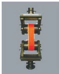
SG-013(#753-141) Max load:200KN Usage: 200mm broadband tensile experiments
